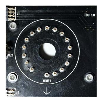
Figure 2–2 Tube socket showing keyed pin
