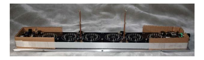
Inspect the small neon lamps (on the copper rods) for any misalignment that may have occurred during shipping. You can carefully reposition the lamps on the end of the rods if needed. If the copper rods are bent, be very careful when trying to straighten them.
