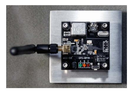
Note: This illustration shows the high-power GPS repeater with external antenna. Older clocks may have the standard GPS repeater which looks similar but does not have the external antenna.
