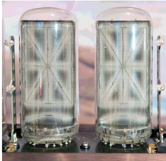
Figure 2-4 Tubes installed in sockets
