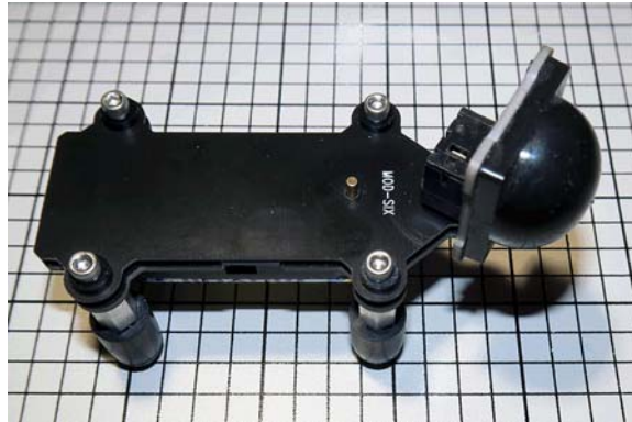
Figure 2–11 MET-PIR top view
