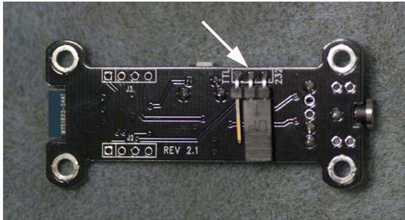
The underside of the TimeLink receiver has a 3-pin jumper with one side labeled TTL and the other side labeled 232. A black plastic Berg jumper connects either the 232 pin or the TTL pin to the center pin. Verify that the jumper on the bottom of the TimeLink receiver is set appropriately for your clock.
