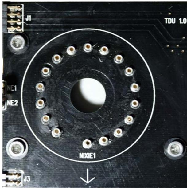
**Caution:** The hole in the circuit board is to accommodate the glass protrusion left over from when the tube was manufactured. That protrusion is one of the most fragile components of the tube, so be careful not to bump it on anything and never stand the tube on a completely flat surface.
