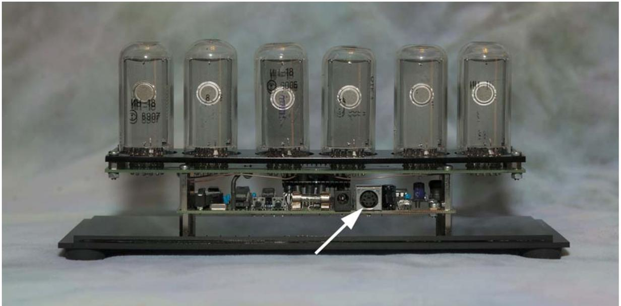
If the clock has an existing GPS receiver connected to it, power off the clock and disconnect the GPS receiver. Re-apply power to the clock and use the clock's setup mode to select the appropriate time zone. You may also wish to set the clock to an incorrect date and time in order to verify that the TimeLink receiver can correctly synchronize the clock. The NCV2.1 clock detects the presence of a GPS receiver automatically and
