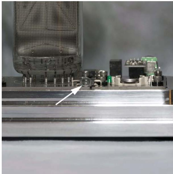
Carefully remove the four clear plastic shipping "bumpers" from the clock, two on the front and two on the back of the clock circuit boards on the left and right black connectors. These are used during shipping to prevent the cover from shifting and becoming scratched. As the bumper is slightly larger than the connector it is attached to, you can simply peel it off by gently pulling on the top edge of the bumper.
