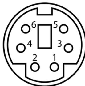
**Caution:** This illustration shows the connector on the clock (socket) side. Pin numbering on the TimeLink receiver cable (plug) side is the mirror image of this diagram.
