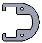
**4.7** Identify the following part. Later versions of the module will only have the one large hole. Place the part so that either both (early versions) or just the central (later version) trimmer on the module is accessible. Access is only required for the central trimmer.
