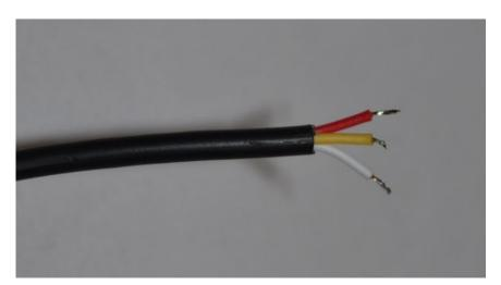
**3.3** Using a continuity meter, identify the GND, 5V and Signal wires, and make a note of which colour wire corresponds to each function:
