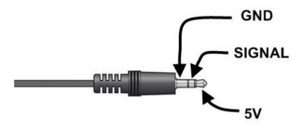
**3.4** Solder the three wires to the pins on the module as shown below, but do not follow the colours below. Follow the note you made earlier as to which colour corresponds to which function.
